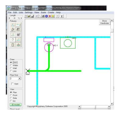
Change the pipe size to 2 and do the same for the "lav" drain pipe.
