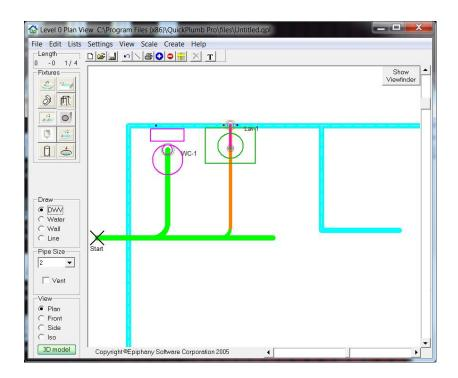
Select "Water" from the Draw Box and add a 1 inch cold water supply pipe. As before, extend it just past the lav fixture. Change the pipe size to ½ inch. Click on each fixture and drag a line down to the 1 inch supply pipe to make the cold water connections.
