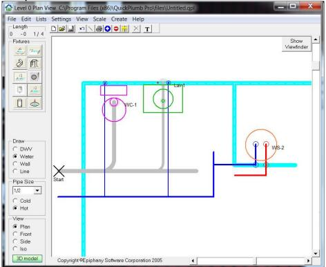
Notice it automatically adds the hot water line. Connect it to the lav.
