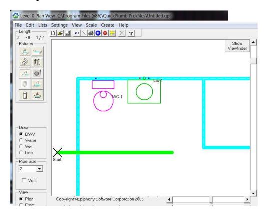
Now draw a vertical line from the toilet waste connector to the building drain.
